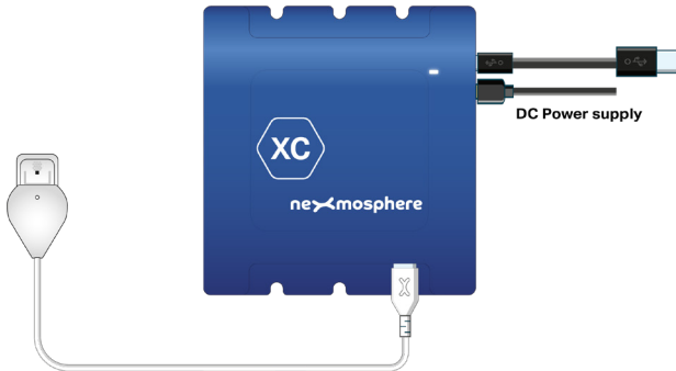
Example connection to XC Controller
