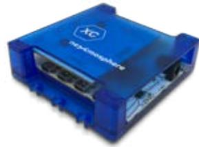
The 700 series is equipped with X-wave interfaces which allow connecting flexible pixel LED strips. X-Wave LED technology allows the user to select one of the numerous pre-programmed animation patterns and modify its parameters to fit the exact application, whether it's a gentle soft glow or a complex running light.
