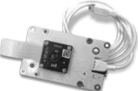
The X-Eye Gender sensor detects the gender and age range of a person. It does not require network connectivity and doesn't store video data, making it 100% GDPR-compliant.
