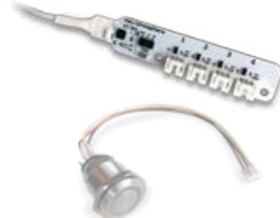
The X-Touch button interface is a 4-channel push-button interface with LED control and can be used in combination with industry-standard push buttons. It allows the connection of up to four buttons onto a single interface. This results in the connection possibility of up to 9 push buttons even on the smallest Xperience Controller. Programmable LED output options are on, off, slow and fast blink.
