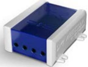
The EM-F Extension Modules receive the signals coming from the P3 sensors after these have been paired with a wireless X-talk interface. Each P3 sensor connects to its own wireless X-talk interface on the EM unit. Combine a maximum of 5 EM units onto the controller unit, allowing up to 40 sensor connections on one single controller. All EM modules only work in combination with an XM Xperience Controller.
