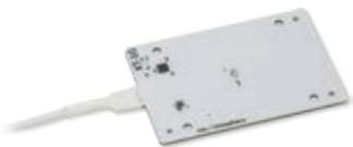
The X-Touch buttons are capacitive and detect a person's touch on the button or an overlying material. The technology works with multiple non-metal overlay materials, such as acrylic, glass, cardboard, and wood. They can be integrated into furniture without visually drawing away from the design. The button sensitivity can be adjusted, and they are available in various sizes and configurations.
