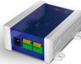
The EM modules define the exact specification of the complete XM Xperience controller. Combine any of the modules into one system to make it fit the exact application needs. Different functionalities such as LED control, audio switching or large numbers of Element connections through X-talk channels can all be combined on a single XM controller. The EM modules are pre-assembled onto the XM controllers at our production facilities.
