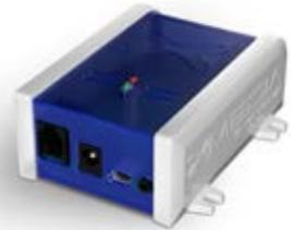
The Modular controllers are fitted with 1 X-talk channel on the unit itself and can support up to 5 Extension Modules and 8 Shop Modules. The Controllers are equipped with a USB or RS232 interface to integrate the sensor Elements with your connected device via our API.
